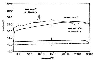
**Figure 7.** DSC curves of **NBD** at heating rate of 20 °C/min under N<sub>2</sub>: (a) first heating, (b) first cooling, (c) second heating, and (d) second cooling.
