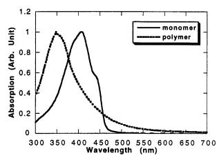
Figure 10. UV-vis absorption spectra of (a) BBD and (b) PBBD in CHCl<sub>3</sub>. Intensities were normalized in order to optimally fit the graphs.
