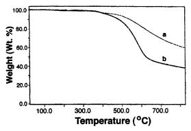
**Figure 6.** TGA thermograms of (a) **MBD** and (b) **BBD** (40  $^{\circ}$ C/min under  $N_2$ ).
