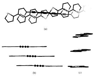
**Figure 4.** (a) View of slipped  $\pi$ -stack (staircase pattern) as seen perpendicular to the molecular plane, showing the alignment of the diacetylene groups and the minimal overlap between the ring atoms. (b) View orthogonal to that in part a and perpendicular to the long axis of the molecules. (c) View along the long axis of the molecule.
