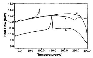
Figure 8. DSC thermograms of (a) NBD, (b) BBD, and (c) **MBD** (20 °C/min under  $N_2$ ).
