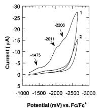
**Figure 13.** CV (100 mV/s) curve of **PBBD** in acetonitrile vs ferrocene/ferrocenium. Curve 2 is a blank run.
