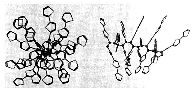
**Figure 11.** One of many possible chain conformations that results in acceptable distances between the side chain substituents. The alkyl groups have been removed for clarity. Views down the chain axis (left) and at a right angle to the chain axis (right).
