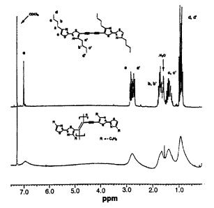
Figure 9. <sup>1</sup>H NMR spectra of (a) BBD and (b) PBBD in  $\widetilde{\text{CDCl}_3}$ .
