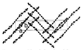
**Figure 3.** View of the molecular packing of **6b** as seen perpendicular to the b axis, showing the  $45^{\circ}$  angle of the molecules to the stacking axis.
