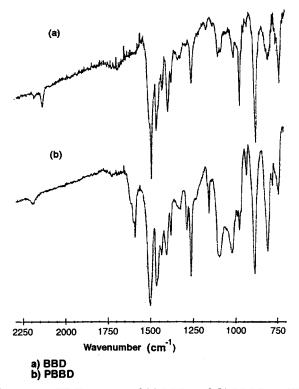
Figure 12. FT-IR spectra of (a) BBD and (b) PBBD on KBr
